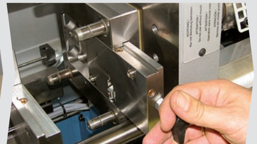
Removable mould inserts for e.g. fast changing / switch
