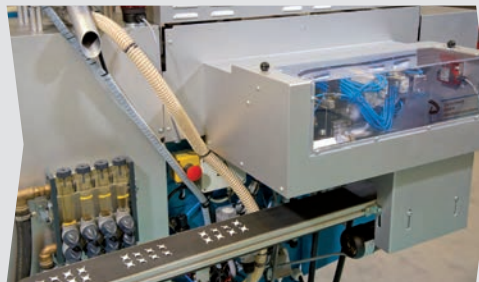
Compact handling for parts removal on the rear of the machine
